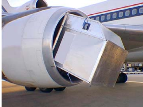
Container blown into engine of L-1011 from adjacent aircraft engine thrust
