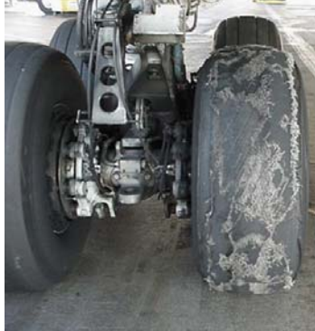
A re-treaded tire that delaminated and left debris behind- airline responsibility
